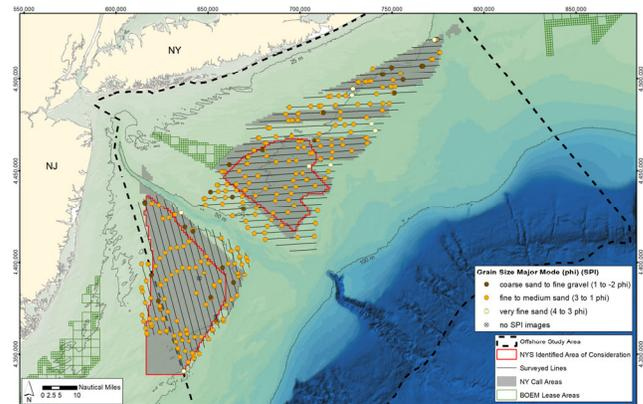
**Figure 7. Map showing MBES lines and grain size results from the 300 SPI/PV station locations occupied during this survey superimposed on areas considered for development.**
