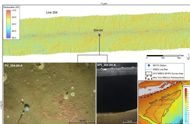
**Figure 8. Data sample from SPI/PV station. Top panel shows a sample of MBES backscatter data, and location of the SPI/PV station. Lower left and middle panels show example plan view and profile view image of the seafloor.**
