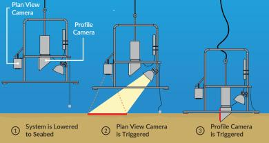
Concept of operation of Sediment Profile Imaging and Plan View camera systems
