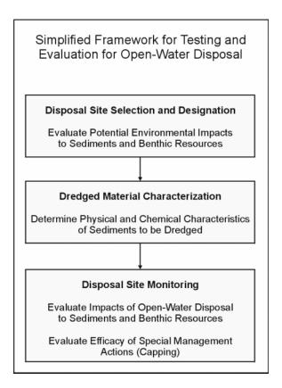
FIGURE 1 Simplified framework for testing and evaluation of dredged material being considered for open-water disposal (adapted from EPA/USACE, 1992).
