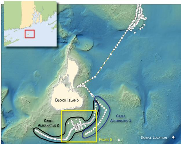
Figure 4. Stations sampled with the Sediment Profile Imaging (SPI) and Plan View (PV) camera system.
