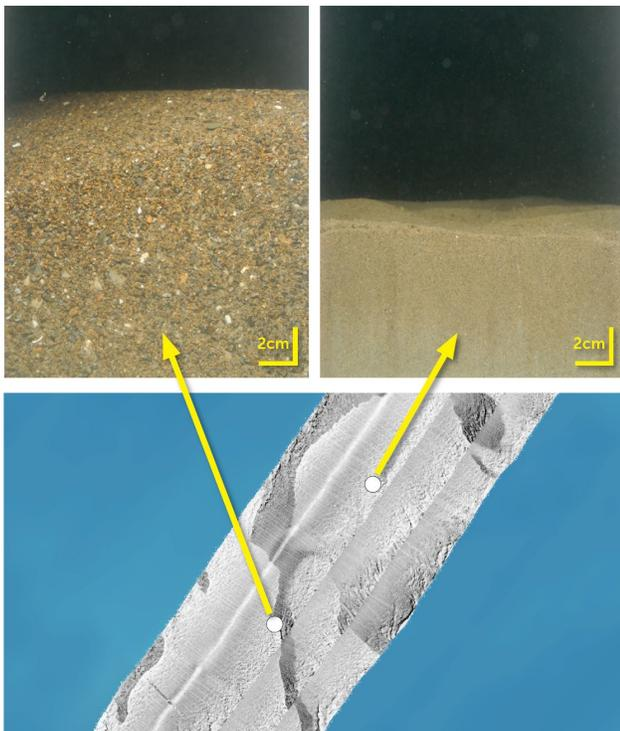
**Figure 3. Use of SPI/PV to ground-truth side scan sonar data.**
