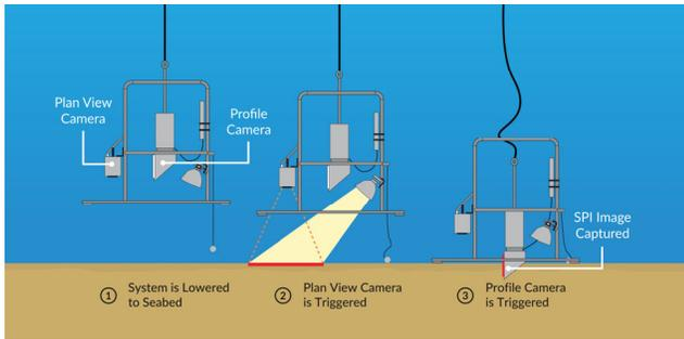
**Figure 2. Operation of Sediment Profile Imaging (SPI) and Plan View (PV) camera system.**
