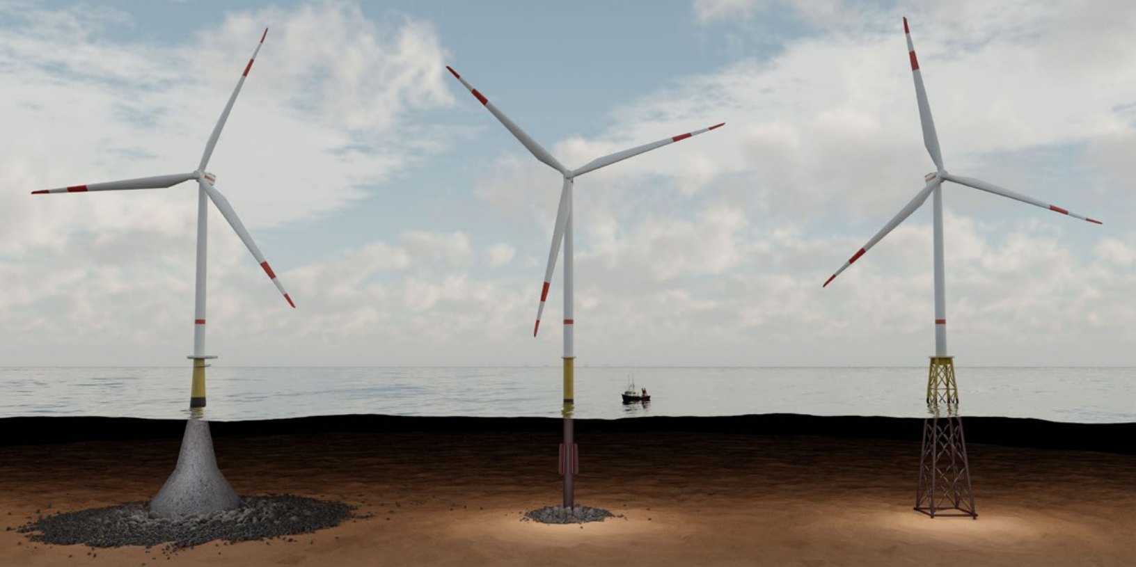
Illustration of gravity, monopile, and jacket foundations (from left to right) © INSPIRE Environmental
