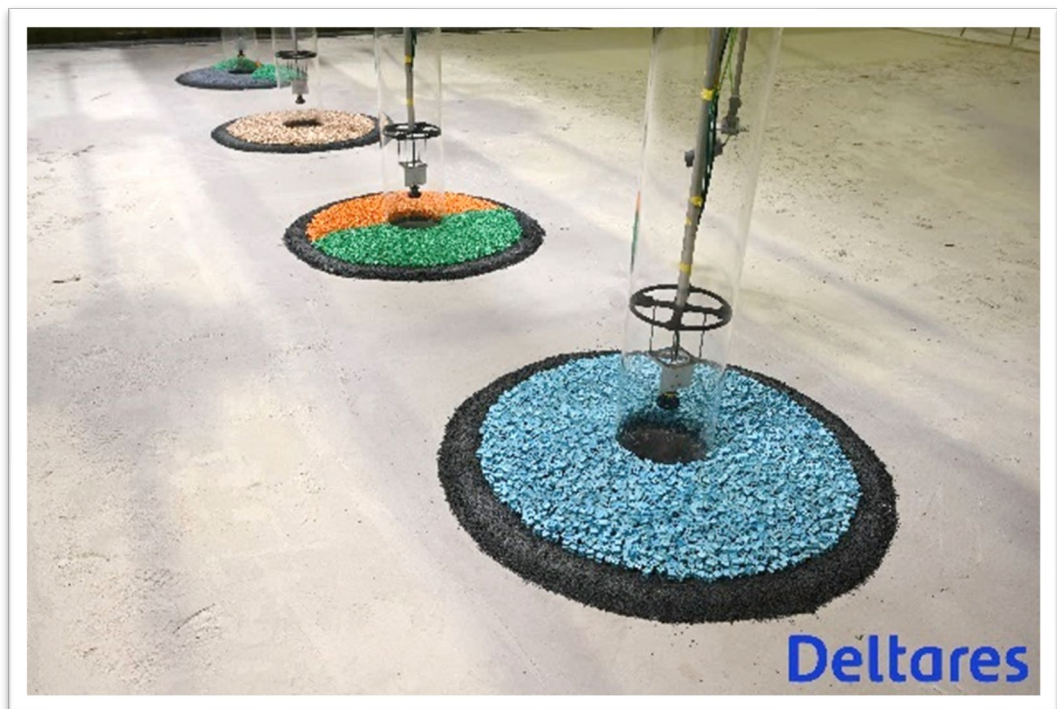
Figure 3-2 - External stability test set-up for JIP SPREE around monopiles (source: Deltares)
